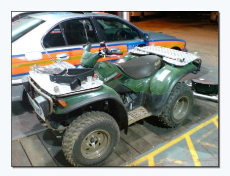
Quad bikes are all not designed for road use and are usually used for tracking whilst filming 'off-road' or in areas where lack of adequate space makes the use of a normal tracking vehicle impossible.
