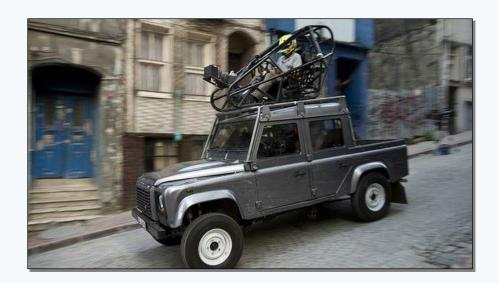
Most POD cars have been adapted purely for film purposes and therefore will **not** always comply with Road Vehicles Construction and Use Regulations 1986 nor Section 41 RTA 1988, meaning it will not be road legal. The Road Traffic Act and construction and use regulations apply to a public road, even one that is closed under a traffic order.
