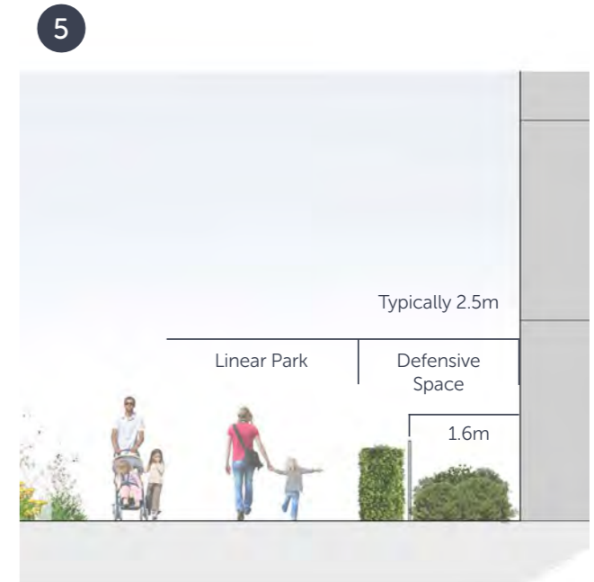
Defensive Treatment 05 Private terraces which interact with the Linear Park are defined with a railing, and hedge planting to the perimeter. Additional planting within the terrace softens the space.
