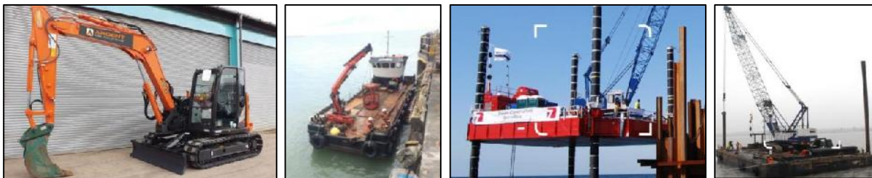
Figure 8: Key Construction Plant (left: Excavator, centre left: multicat, centre right, Haven Seajack (JUB), right: Haven Seaforth (Crane Barge). Source: RED7MARINE RAMS versions R7M-520038-MST-003 and-R7M-520038-MST-001-Construction Sequence
