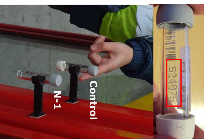
The above picture shows the first sampling tube and the control tube in place on the school ground
