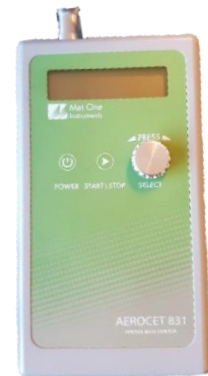
Figure 2: The equipment used to measure PM 2.5 and PM 10
