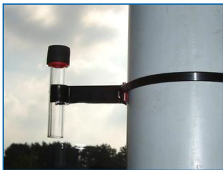
Figure 1: An example of a diffusion tube, mounted to a lamppost
