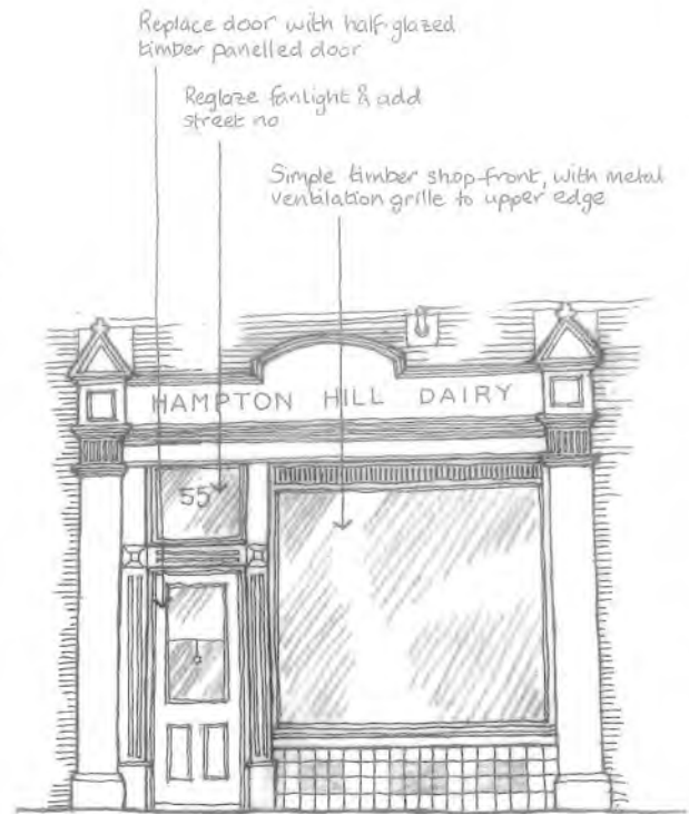
No. 55: Retain stucco pilasters, cornice, fascia and door surround. Replace shop-front as illustration, replace stallriser with ceramic tiles.
